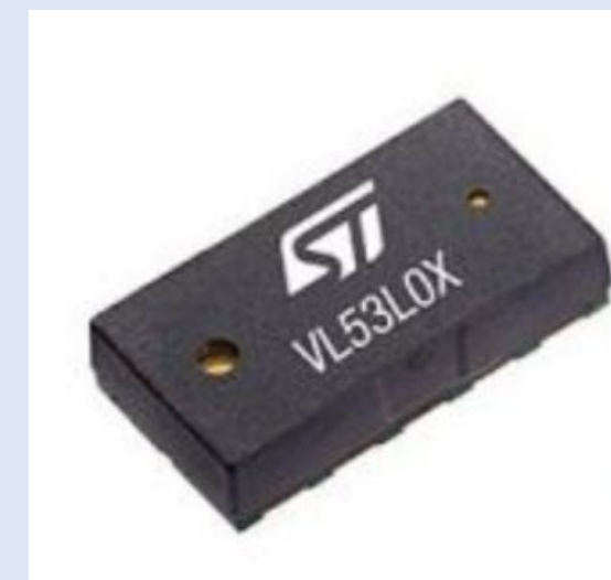
Figure 2.(a) Adafruit GEMMA v2 - Miniature wearable electronic platform (b) VL53L0X Time-of-Flight Sensor
