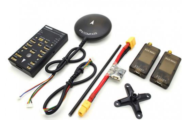
HKPilot 32 PixHawk, GPS Module, and RF Telemetry Set
