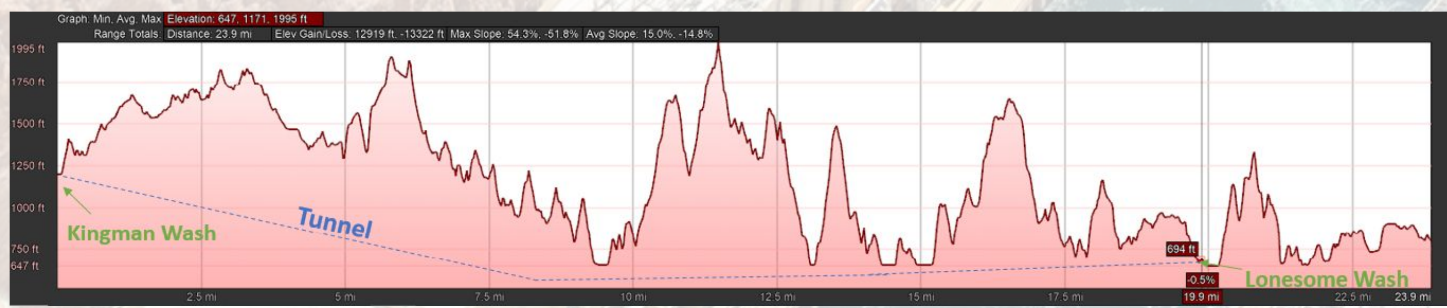
Figure 3. Profile of the tunnel pipeline
