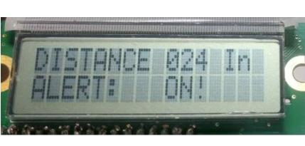
Alert the user of an object that is less than 30 inches away from the sensor.
