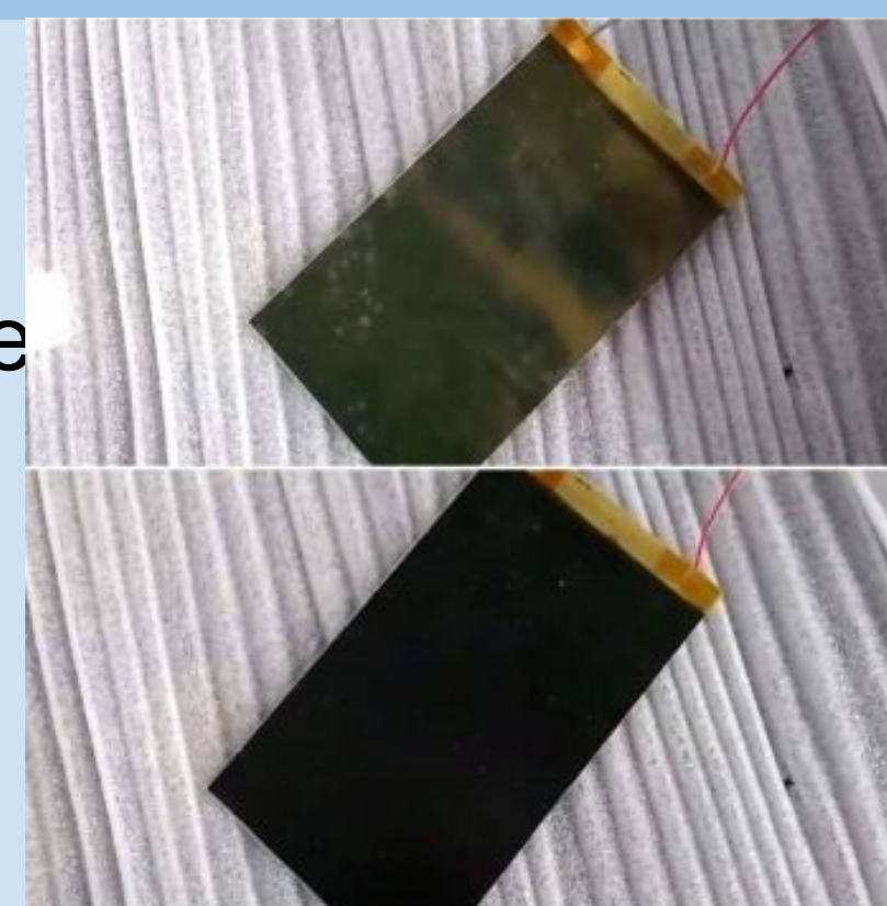
Figure 4: Variable emissivity sample changing in response to solar radiation
