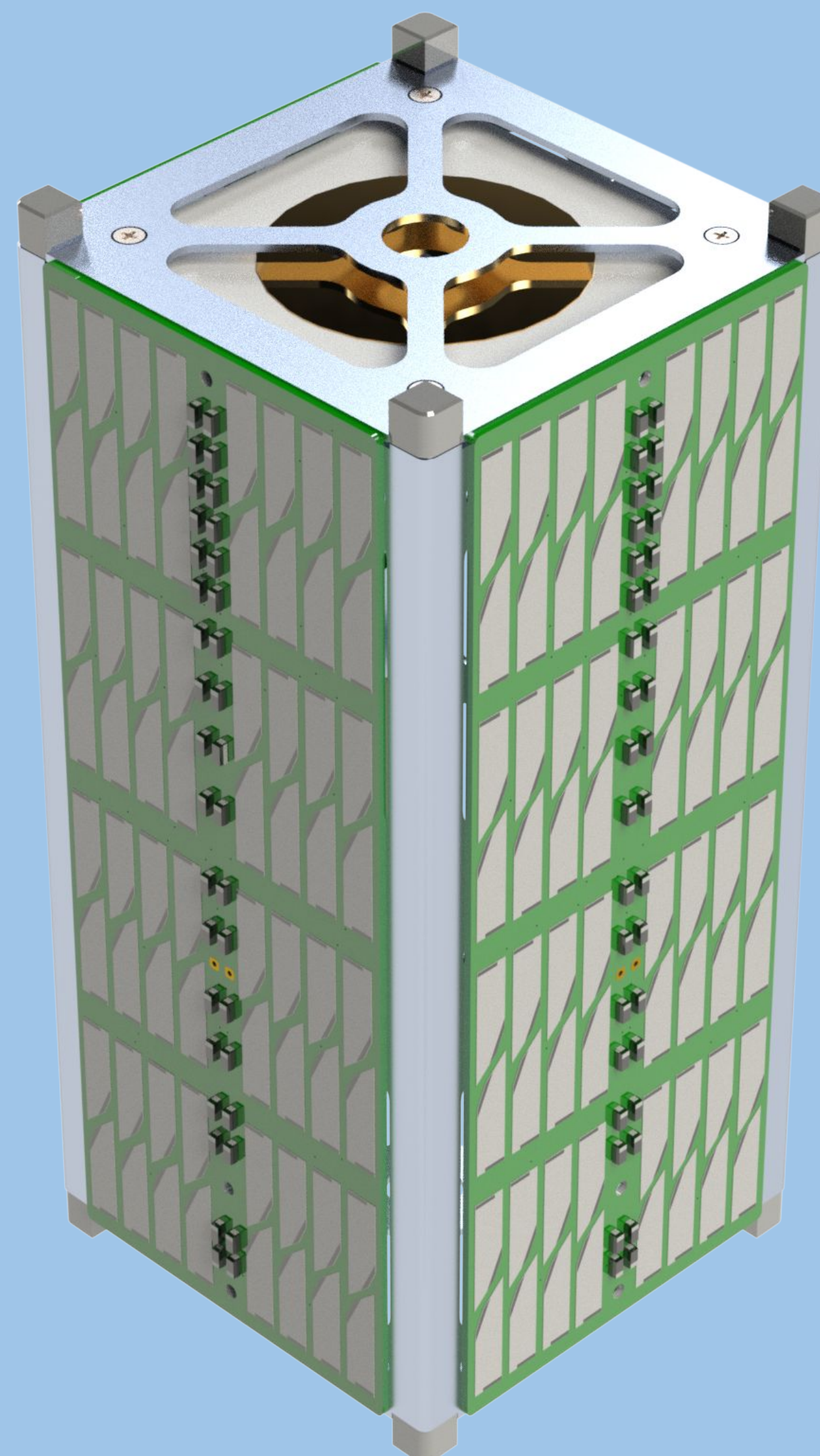
Figure 5: Preliminary SolidWorks model of AntSat 01
