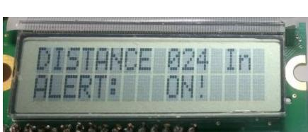
Alert the user of an object that is less than 30 inches away from the sensor.
