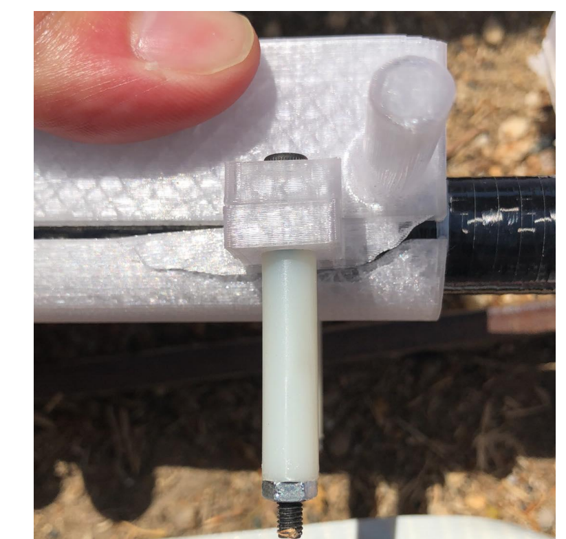
Figure 3. Wing attachment post-test flight showing a crack.
