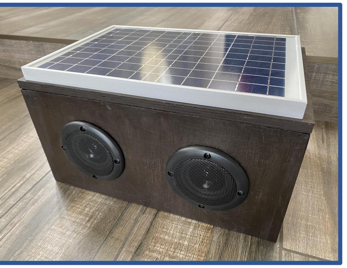
The device is hardwired to a network for initial configuration. We built a landing page that guides the user through its initial setup which connects it to the user's wireless network. Once connected the user can use any browser enabled device on the same network to connect to the speaker.
