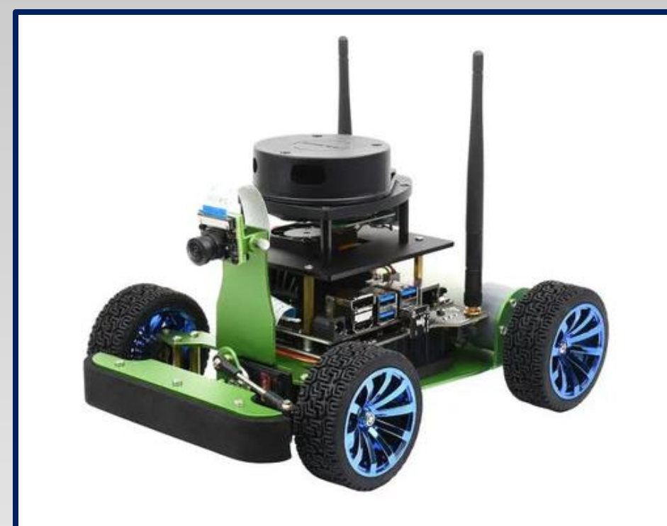
Figure 1: Our project robot: the JetRacer Professional ROS Kit.
