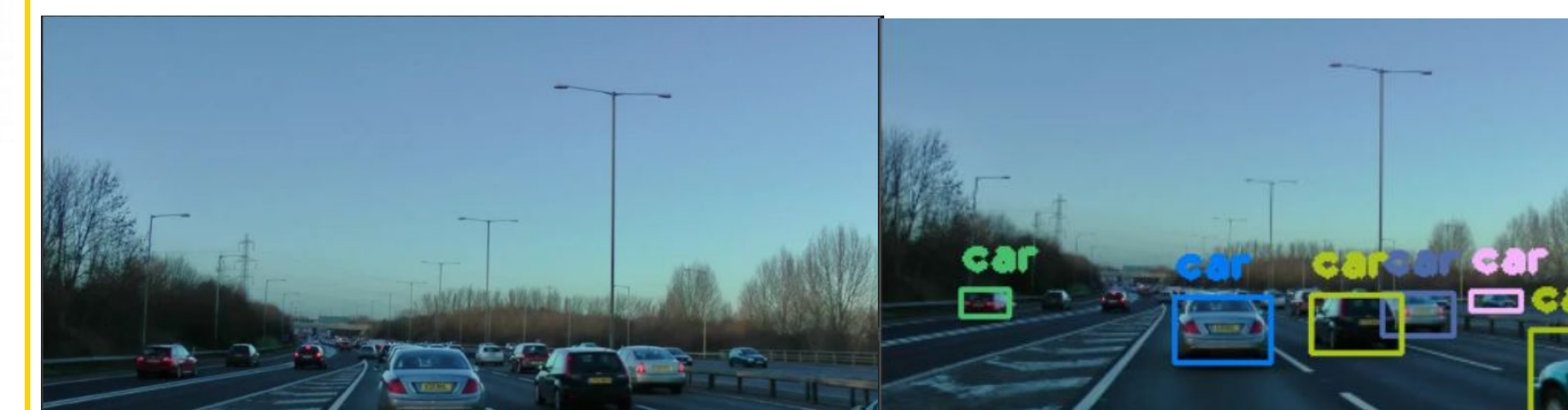
Figure 4 & 5: Using a photo of traffic on a highway as an example, the YOLO algorithm is able to detect multiple cars within the frame.
