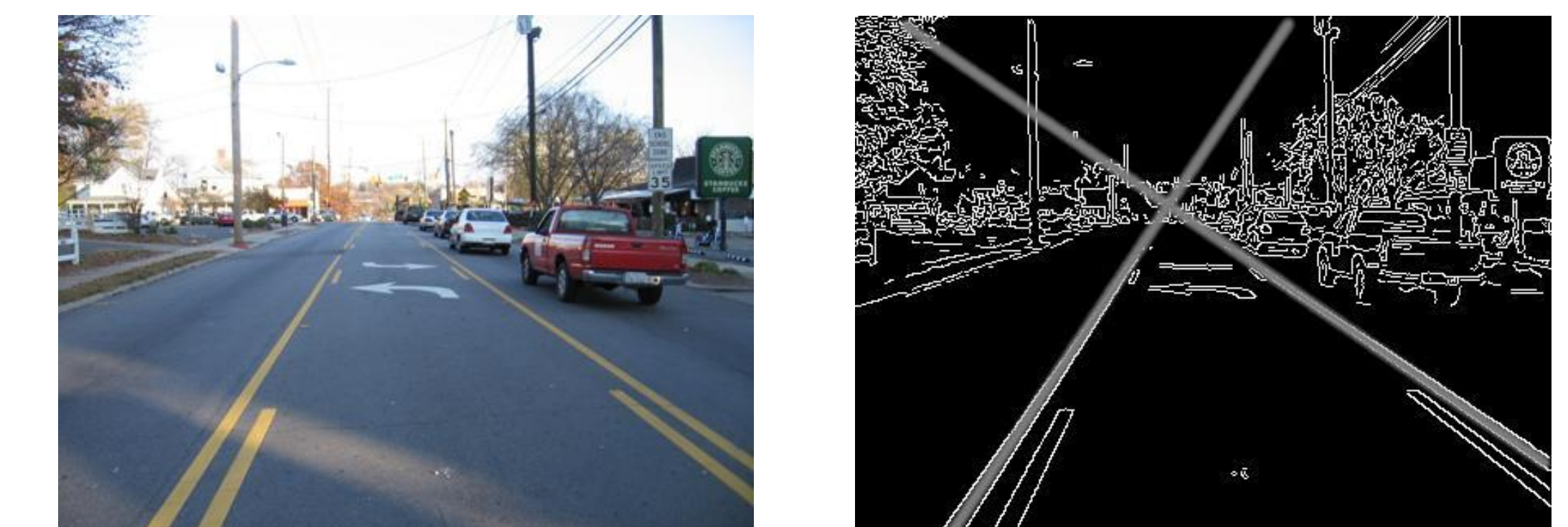
Figure 2 & 3: The black and white image is the processed output from the Jetson. The lines are drawn to match what the program output.
