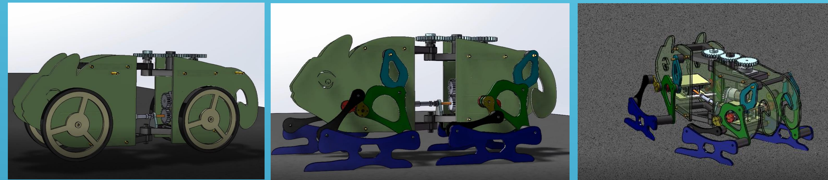
Figure 8: CAD simulations of Steerable Walker with wheels and legs
