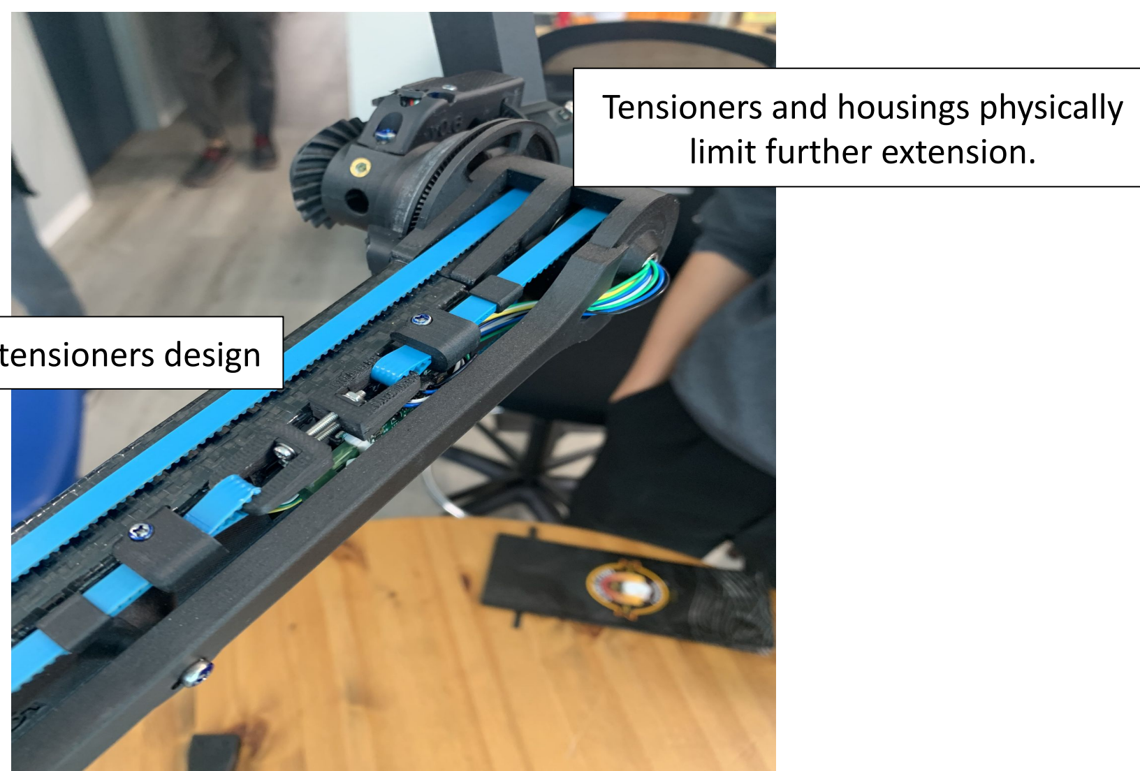
Figure 1. Previous tensioning system physically limited extent of belt movement.
