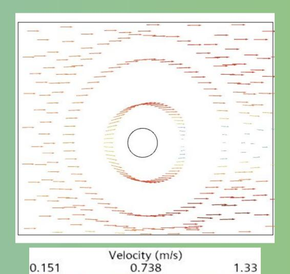
**Computational Fluid Dynamics (CFD) to represent air** flowing through cylinder at 5 m/s Looking Ahead **Proof of Concept**
