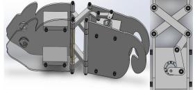
**Mock Model:** Cardboard model of hinge to chassis assembly were made to test and verify for design feasibility and to estimate the size of the steerable walker.
