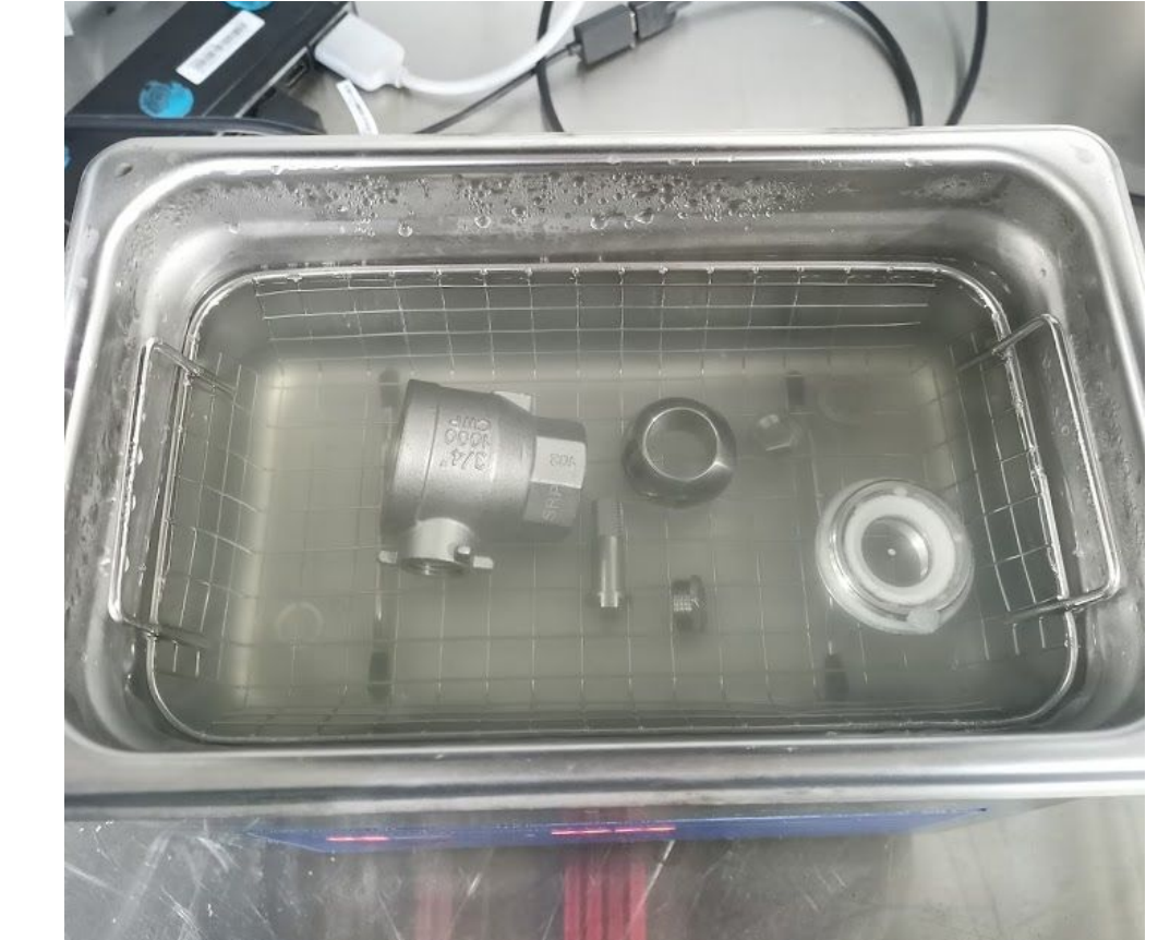
Cleaning ball valve components with isopropyl alcohol in ultrasonic cleaner.
