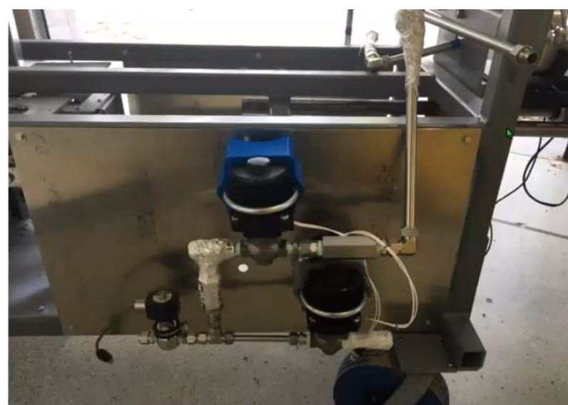
Previous solenoid valve design with the top valve being the main valve
