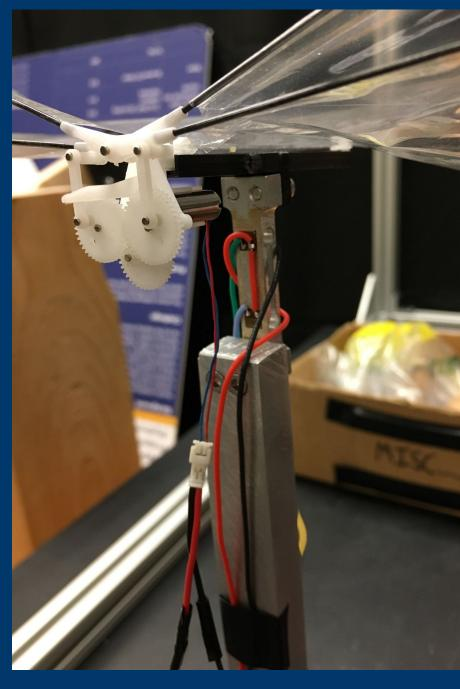
The System Identification and Visualization Team collected thrust and lift data using a high precision load cell to detect small force fluctuations. This data was sent through a hardware filter, amplified, and sent to a DAQ where it was processed electronically. The FFT was then taken to analyze the dominant peaks of the flapping mechanism at varying operation frequencies.
