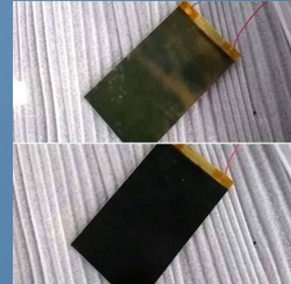
Figure 2. Variable emissivity sample changing in response to solar radiation.
