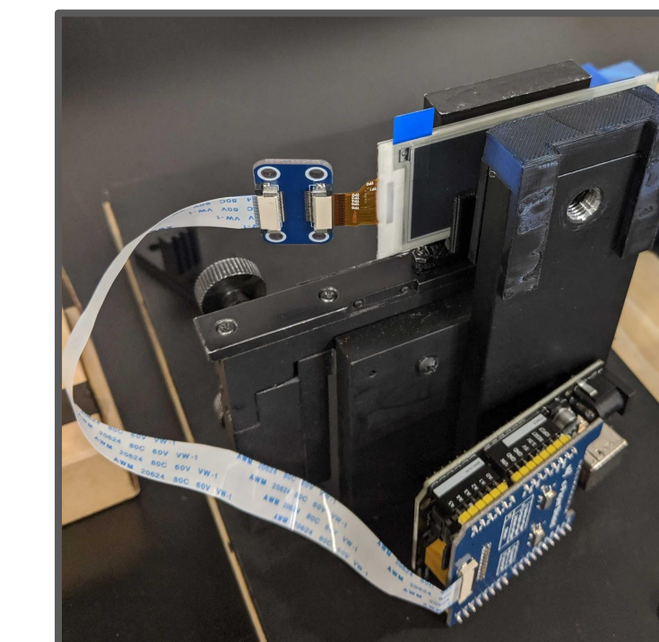
Fig 7: Emissivity testing set up for the E-ink team
