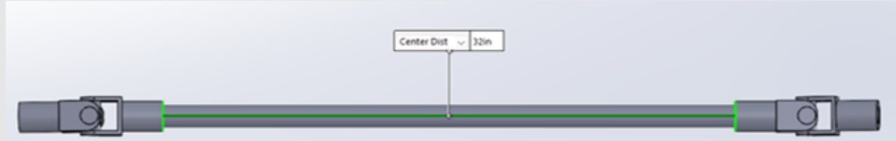
Figure 8. Chromoly Steel (4130) Shaft 1.25" Diameter, 0.083" Wall
