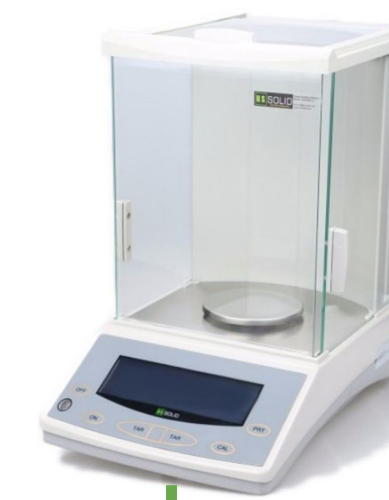
◀ Fig. 5: USS-DBS8 Analytical Laboratory Balance used to weigh dispensed P-32-HA radioactive powder
