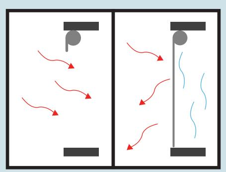
Utilization of shades to regulate building temperature
