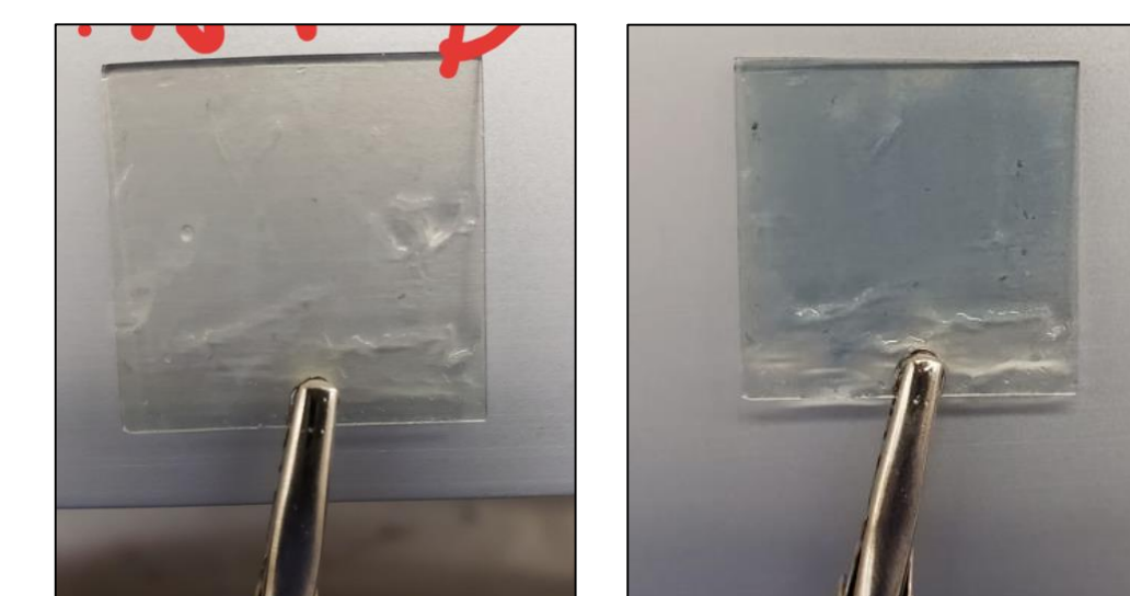
Figures 8 (Left) & 9 (Right): Tungsten Slides Bleached (Left) and Darkened (Right) at 1.75 Volts
