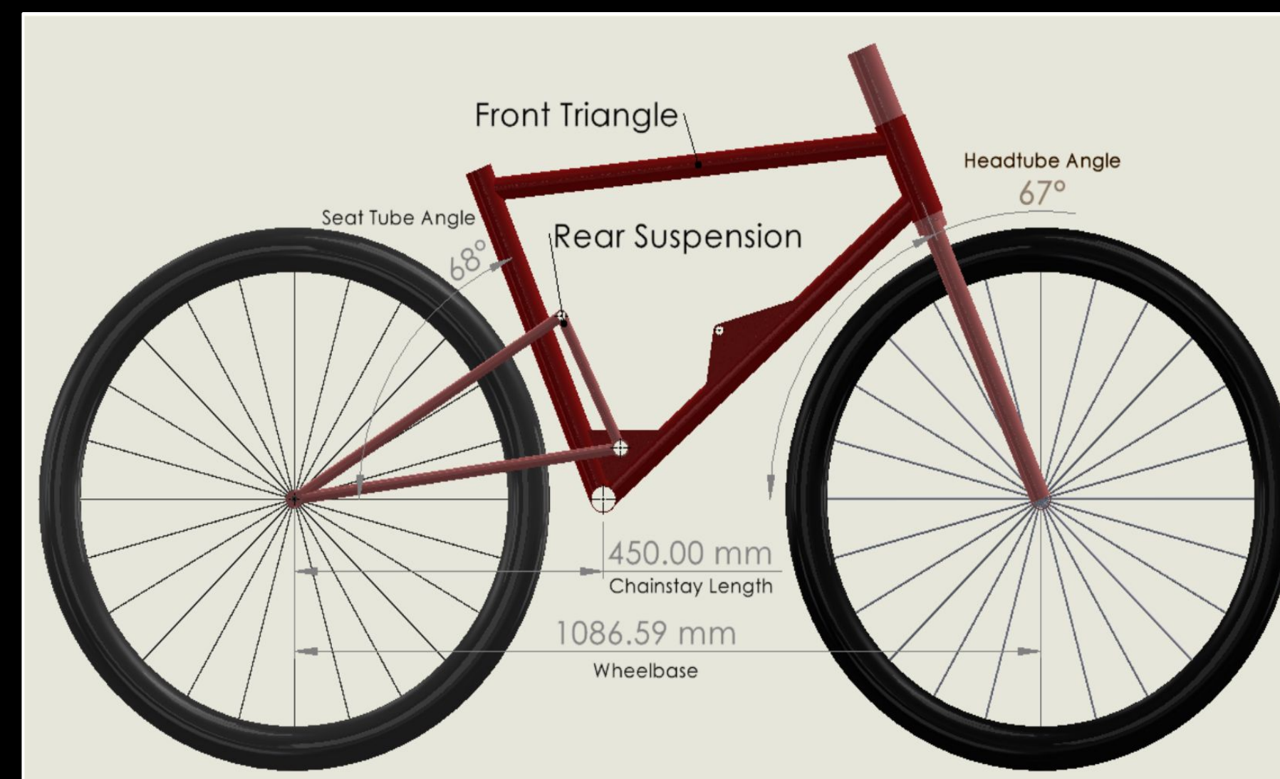
Fig. 2 Bike Nomenclature and Dimensions
