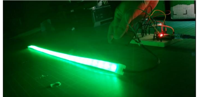
Fig. 4. MaRker Prototype demonstration using a two-meter long NeoPixel strip. The device held in the hands is the FSR to activate the module.
