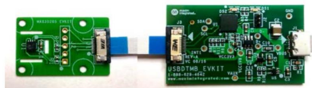
Fig. 3. The MAX30205 evaluation kit in its off state, connected to its controller PCB. The MAX30205 has a metal electrode underneath the image shown which is used to take data. The 10-pin flex cable interfaces the controller to the sensor and the controller provides a I2C to USB interface. This image is property of Maxim Integrated.
