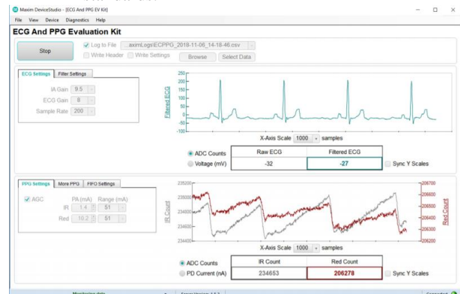
Fig. 7. Device Studio showing an example of the MAX86150 being evaluated and producing an ECG and PPG plot. We have the option of plotting raw or filtered ECG while logging both. The screenshot is property of Maxim Integrated.
