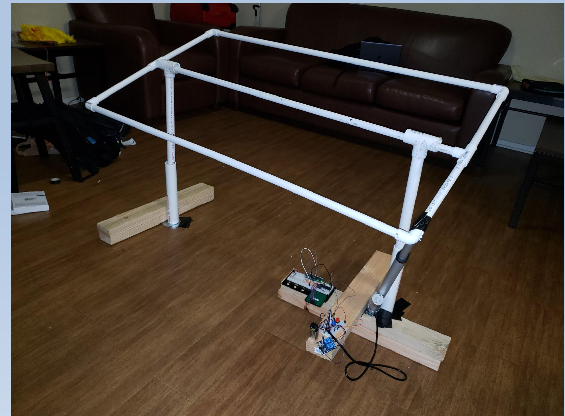
Fig. 3 Prototype for single axis predictive solar panel
