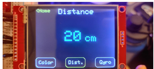
Fig. 9. Distance measurements displayed on the LCD that ends up being attached to the glove.
