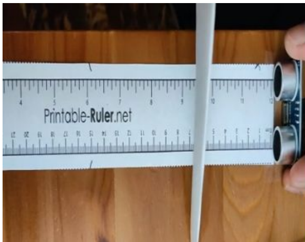
Fig. 7. Testing the distance sensing capabilities of the Ultrasonic using a printable ruler as reference. The ruler's bottom scale is centimeters.
