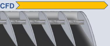
Preliminary CAD model of the morphing wing with inner tensegrity mechanism created using SolidWorks
