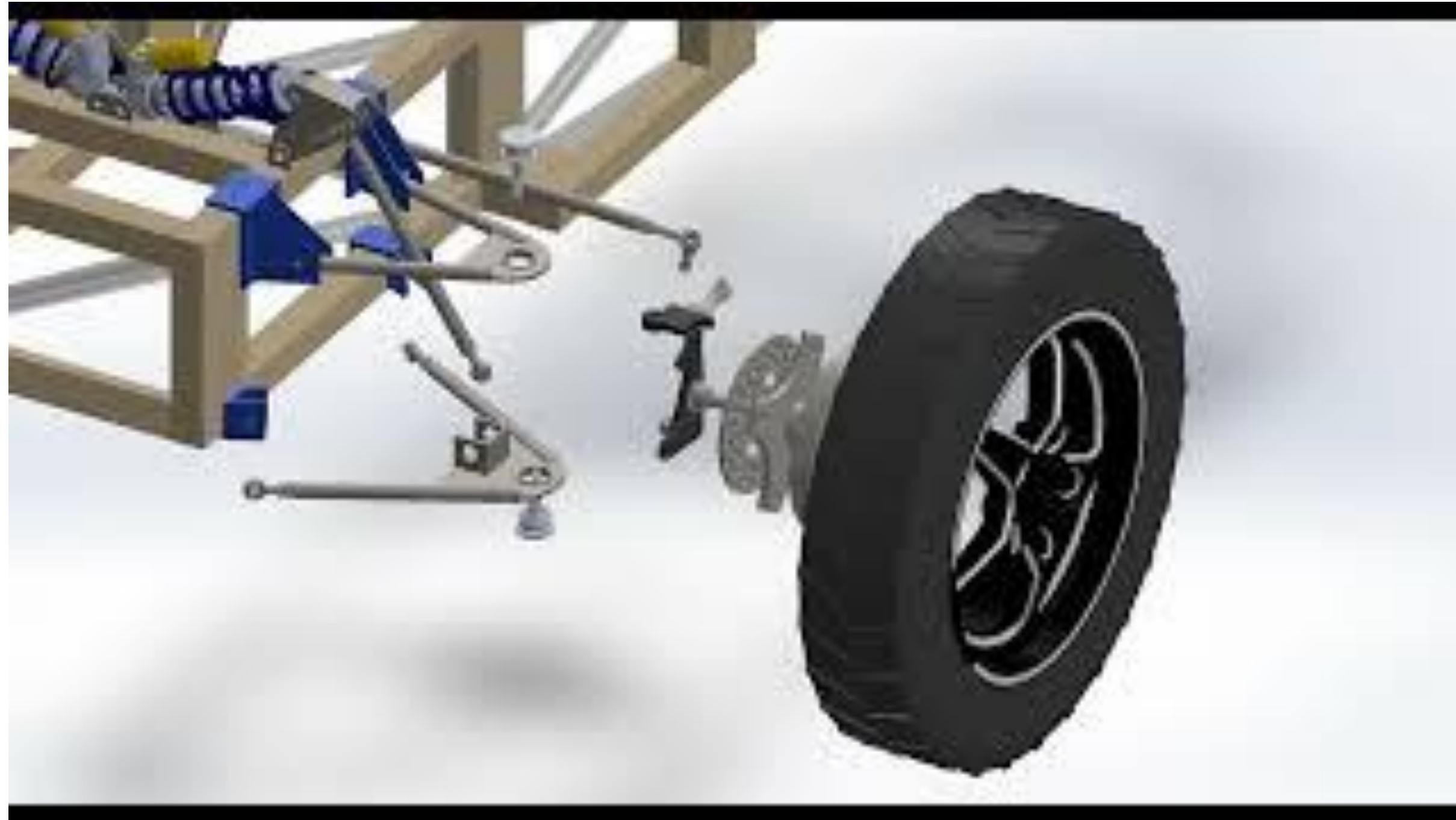
Collapse view of control arm and wheel mounting.
