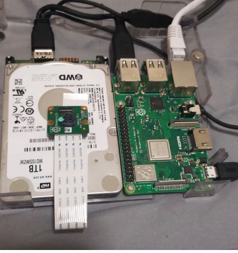
Fig. 2. Our Raspberry Pi 3 Module with the Serial Camera
