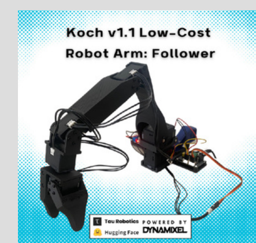
Fig 1. Koch v1.1 Robot Arm $237 Low Fidelity 4 DOF
